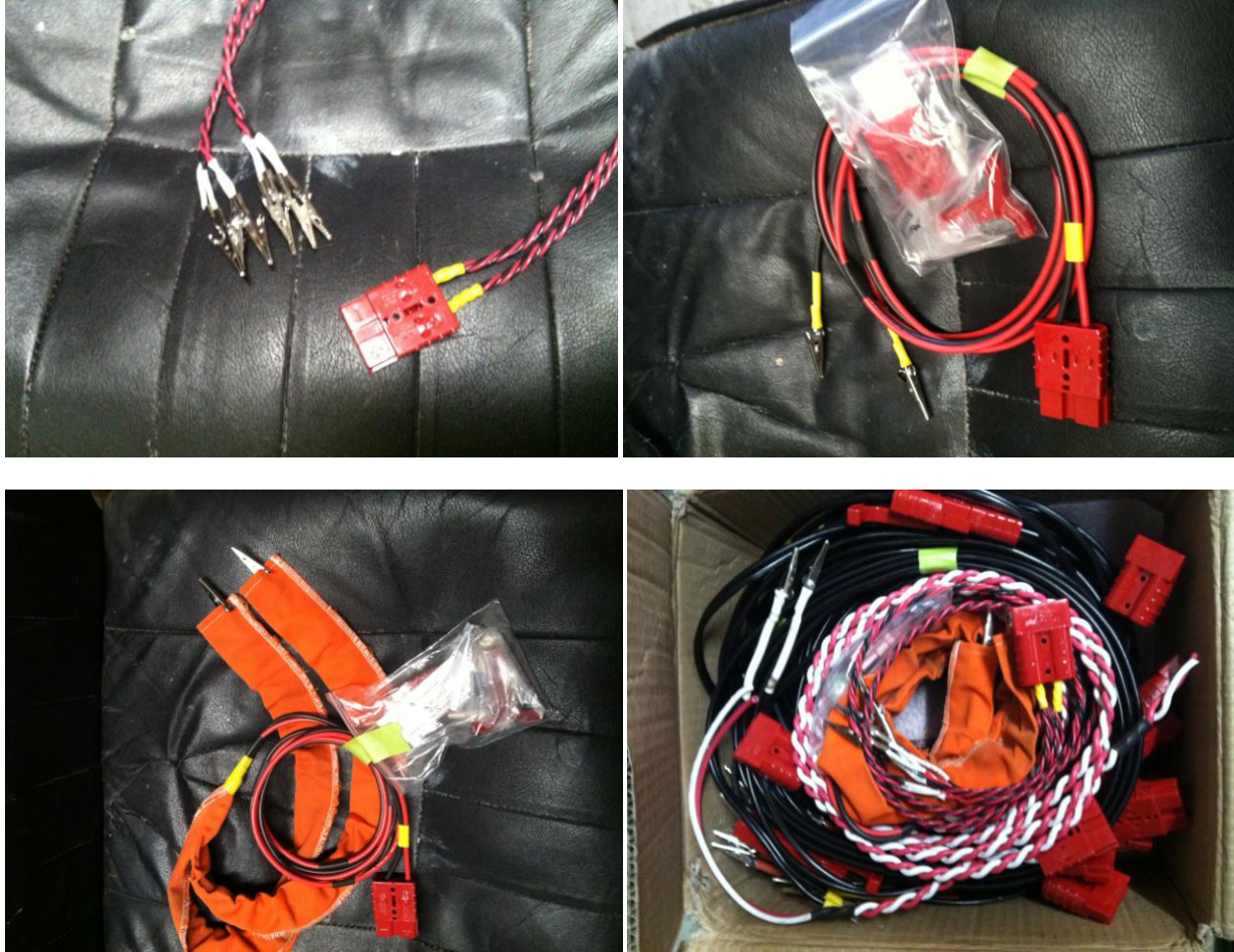
Top-Left: 4-Motor cluster Igniter leads (4'), Top-Right: 6' Deans Ultra-Wire Leads
