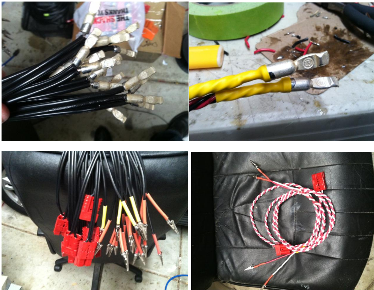
Top-left: soldering SBS-50 terminals to 10GA, Top-Right: Completed SBS-50 Quad lead and heat shrink Bottom-left: 12 Igniter leads with SBS-50 connector, Bottom-Right: Dual 6' Umbilical cord (Model Pads)
